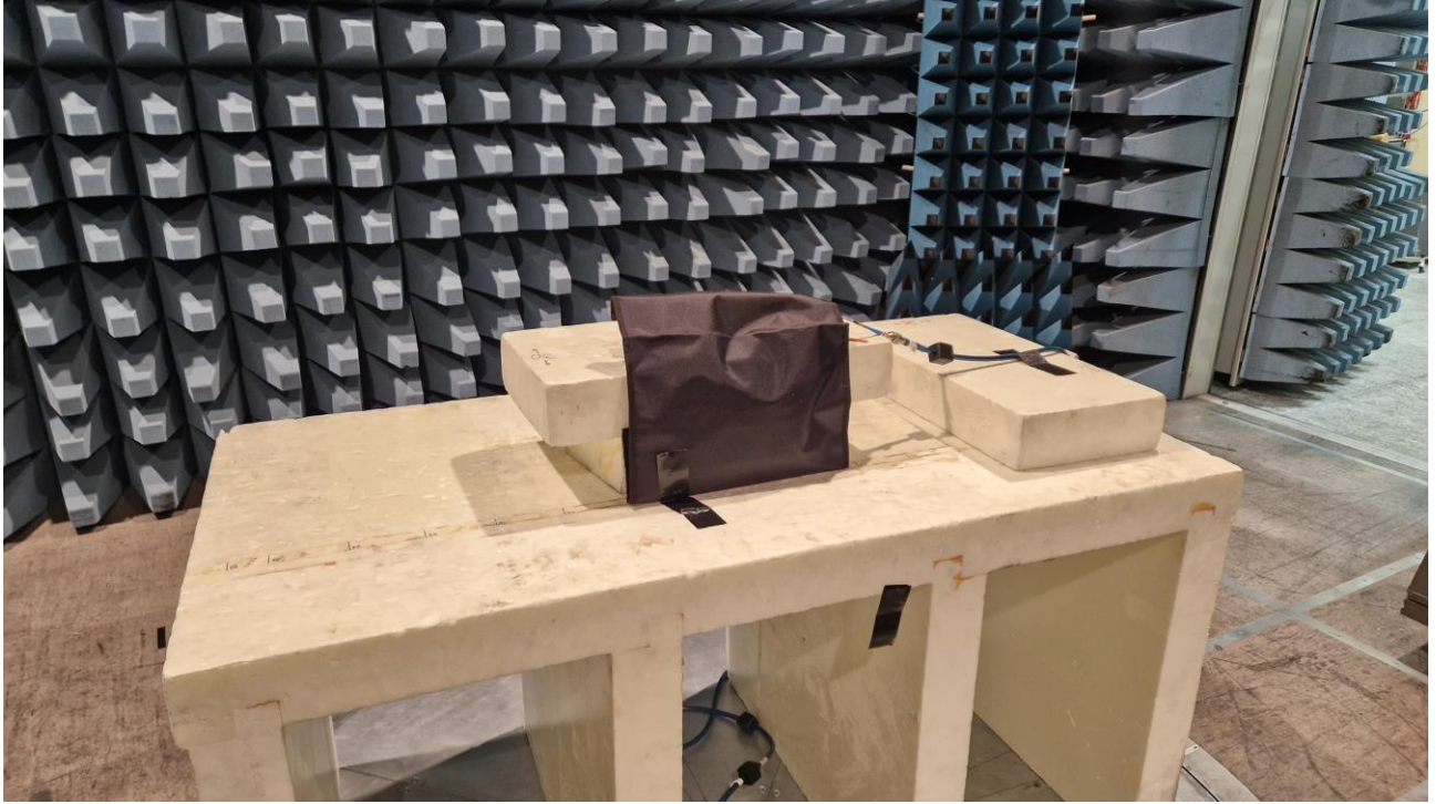
Photo 7. RF Shielding effectiveness test setup, big bag
