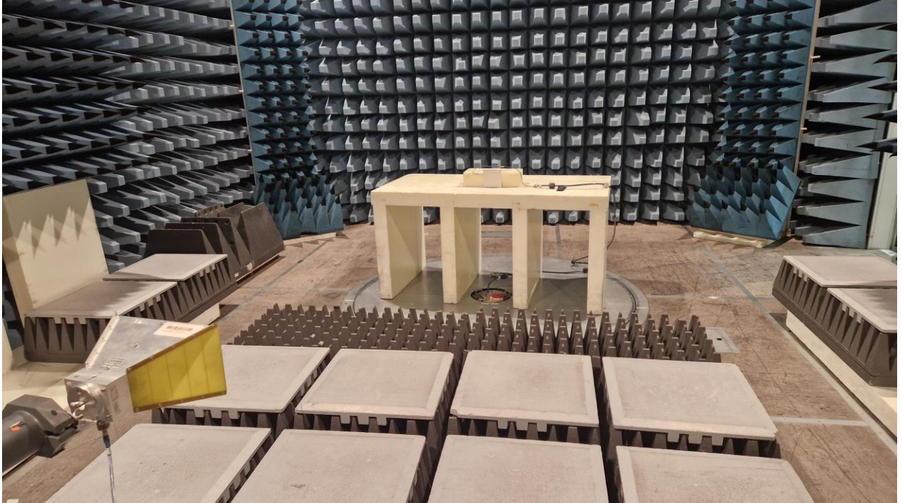
Photo 5. RF Shielding effectiveness test setup, reference measurement
